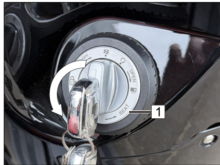
1. With the key(1) in the "LOCK" position, turn it counterclockwise to open the seat (2).
